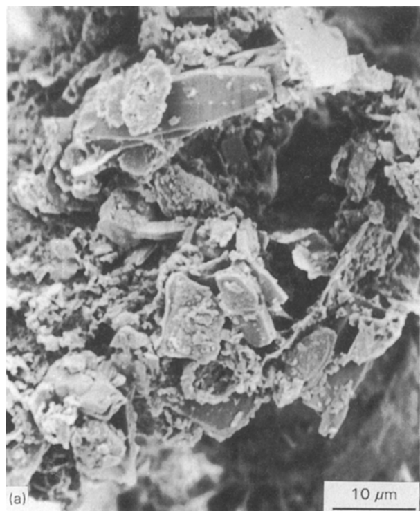
Figure 9 SEM micrograph of representative samples: (a) m5 sample, \times 1500 magnification; (b) m2 sample, \times 3000 magnification; (c) m8 sample, \times 2200 magnification and (d) m4 sample, \times 2000 magnification.
